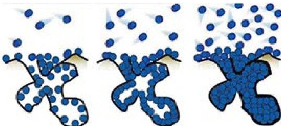
Fig. 2.5: Physical adsorption of gas molecules inside the pore cavities by gradually increasing the applied pressure (from left to right).
