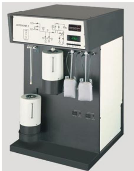
Fig. 4.4: The volumetric gas sorption analyzer Autosorb 1-MP by Quantachrome Instruments; measuring station, vacuum cold trap and two de-gassing stations (from left to right) [71].
