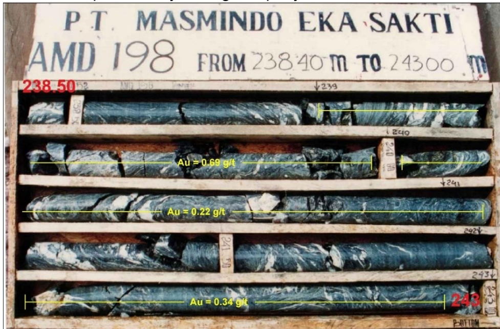
Fig. 37. Borehole photograph of AMD198 at Awak Mas showing thin quartz veins (generally less than 10 cm) within a thick layer of carbonaceous phyllite. Gold-silver grades are based on fire-assay analyses and are provided by the mining company.
