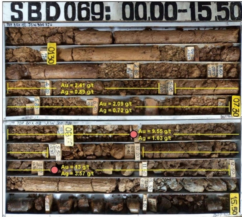
Fig. 36. Bore hole photograph of SBD069 at Salu Bullo showing intense surficial oxidation near the surface. Some samples have a high gold grade with assays up to 13 ppm. The pink circles show gold content > 5 ppm. The yellow bar indicates the samples interval. Gold-silver grades are based on fire-assay analyses and are provided by mining company.
