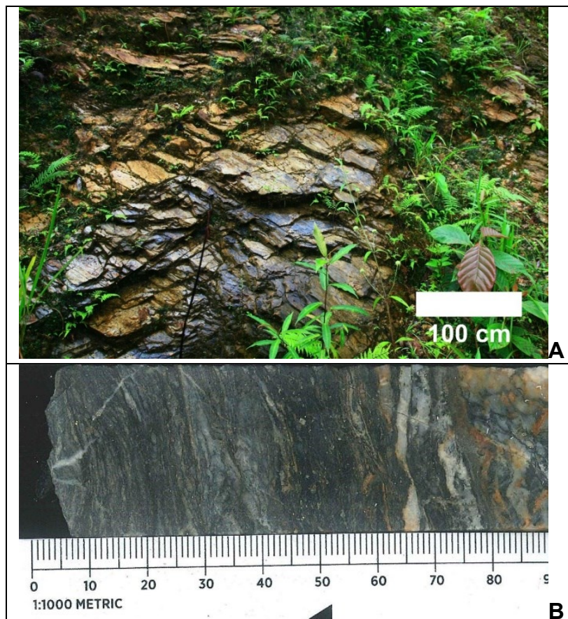
Fig. 23. Photograph of phyllite (A) Field photograph at Awak Mas (courtesy of Agus Haris Widayat). (B) Borehole photograph of phyllite.
