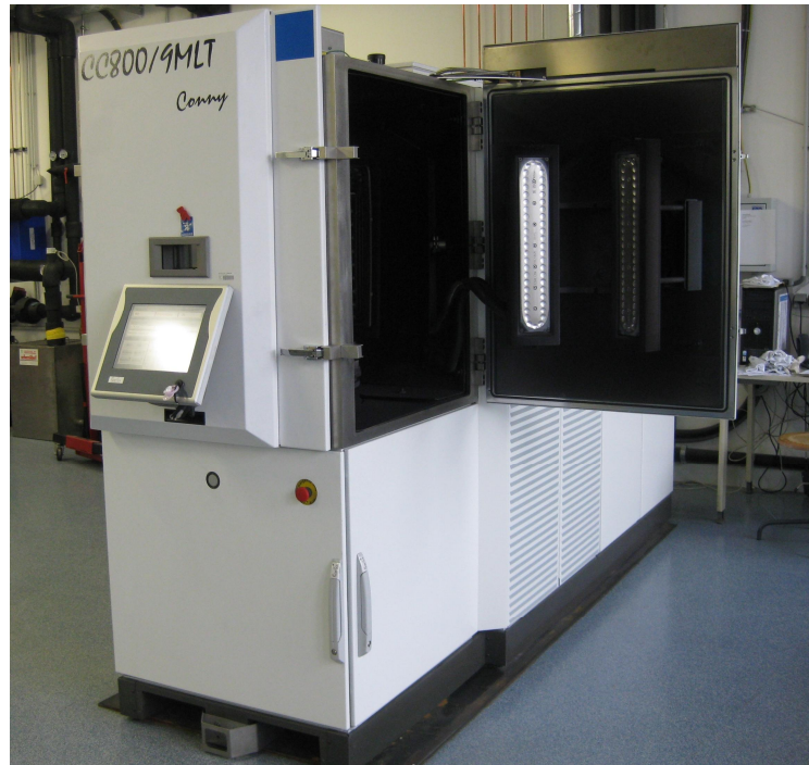
Fig. 6.2: Picture of the industrial scale sputtering device CemeCon CC800 ® /9MLT at the University of Leoben.
