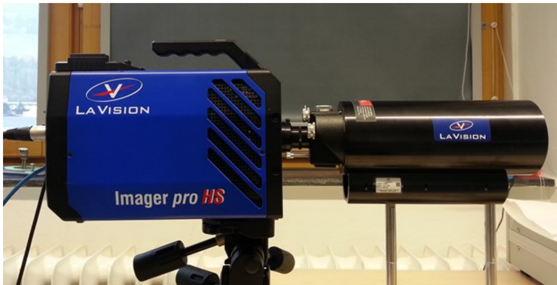
Figure 3-6 The Long distance microscope (right) with a high-speed camera imager Pro HS 4M (left)
