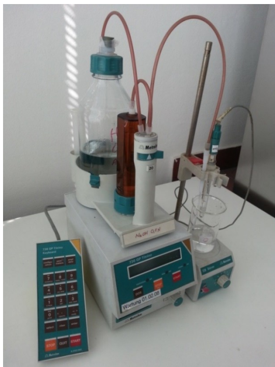
Figure 3-9 The complete set up of automatic titration unit (Titrimo GP 736) and the combined pH glass electrode.
