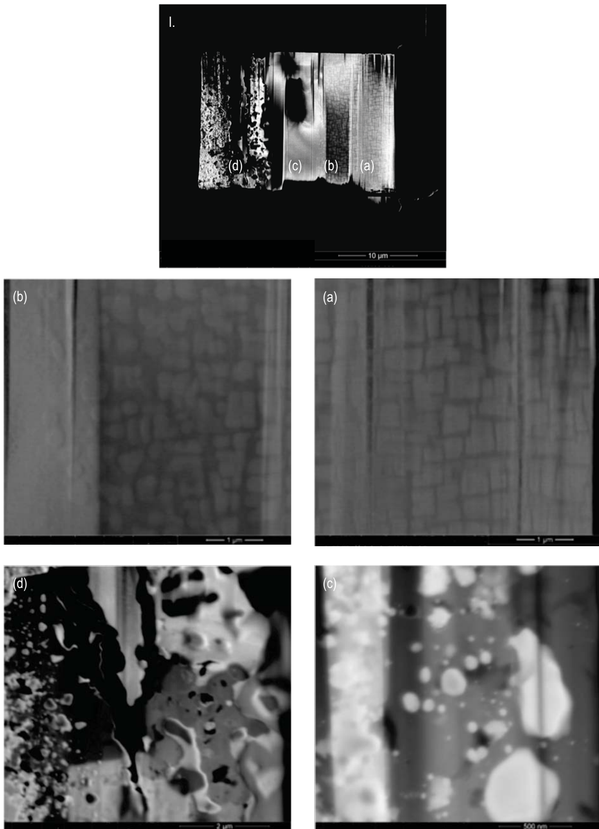
Figure 37 STEM foil of H1560 (I) displaying different stages of oxidation. The numbers do mark areas in the bulk material depending on their state of oxidation. Area (a) of H1560 is magnified on the right hand side. It can be clearly seen that the microstructure is not yet affected by oxygen. Areas (b) to (d), do show the stages of oxidation of the bulk material. While in Area (b) first signs of disorder do already take place, Area (c) displays and disordered state of the material. In area (d) the material suffered severely due to oxidation.
