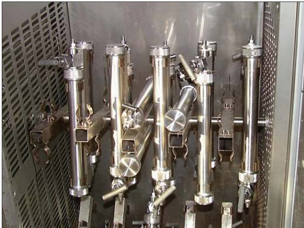
Figure 18 – Autoclaves installed on the wheel in the heating cabinet.
