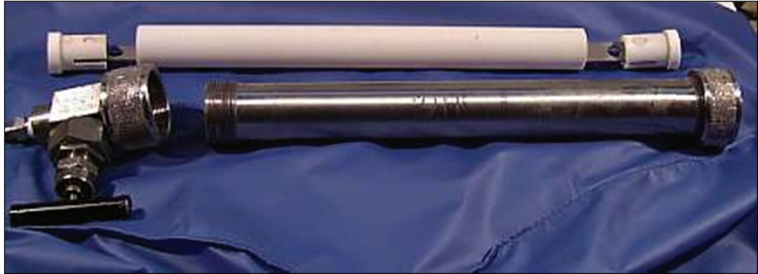
Figure 19 – Samples in Teflon arrangement and autoclave.
