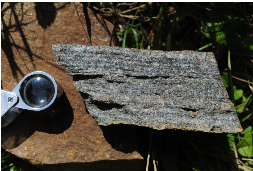
Fig. 15: Hand specimen of biotite gneiss showing mm-scale metamorphic layering and foliation
