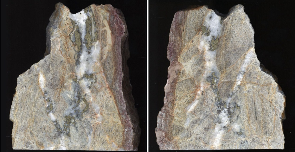
Fig. 50: Ore sample (slabs) from the Barbara dump. Carbonate-quartz-sulfide veinlets crosscut the strongly altered host rock. Frame width 9.5cm
