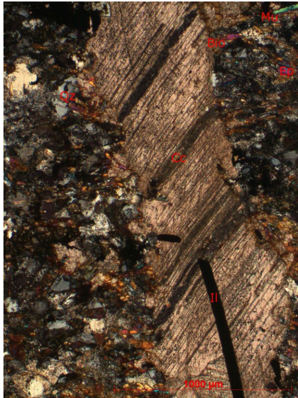
Fig. 49: Veinlets filled with calcite (showing deformation twinning) in altered host rock. The latter contains quartz, calcite, epidote, tremolite(?) as alteration minerals. Sample: 11Sch22a; crossed-nicols
