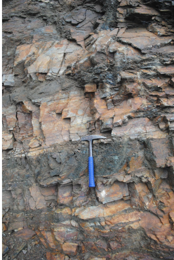
Fig. 13: Alternating sequence of lighter biotite gneiss and darker amphibolite; 1km E of Stadloberhütte WP 88
