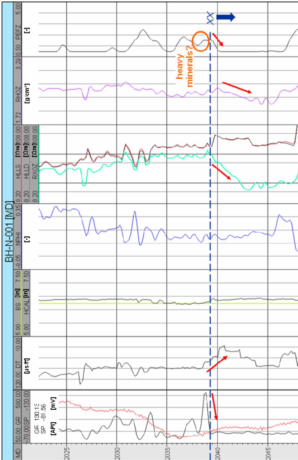
Fig. 57: Correlation of well logs of BH-N-001; the dashed blue line indicates the top of the crystalline basement (Top-XX); The values for GR and SP at Top-XX are displayed on top of the logs (130.13 API, -81.56 mV).
