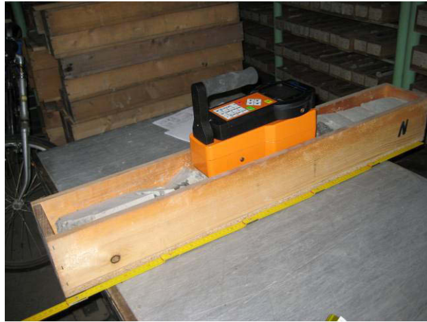
Fig. 32: Measurement of Core-GR, Gamma Surveyor Compact/GF Instruments
