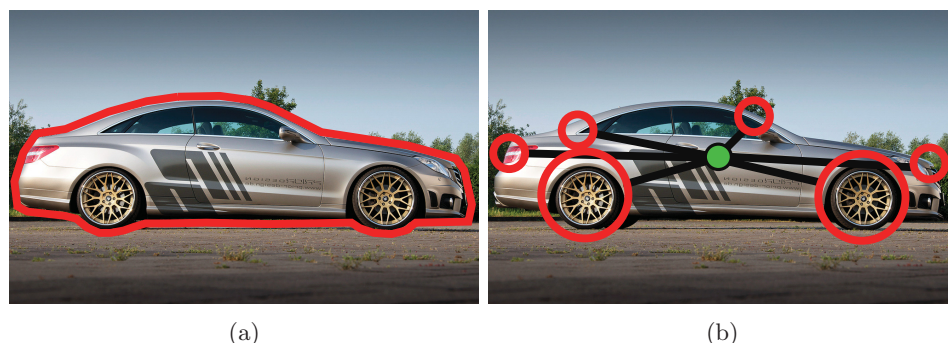
Figure 2.4: (a) A target object and its marked boundary (image source [90]). (b) A part based model which stores the spatial configuration of important parts to the object center (star model).
