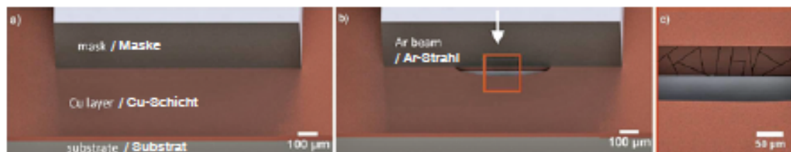
Figs. 2a to c: Broad ion beam cross-section preparation of a thin film on substrate.
