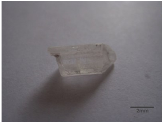
Fig. 21 Single crystal fused magnesia
