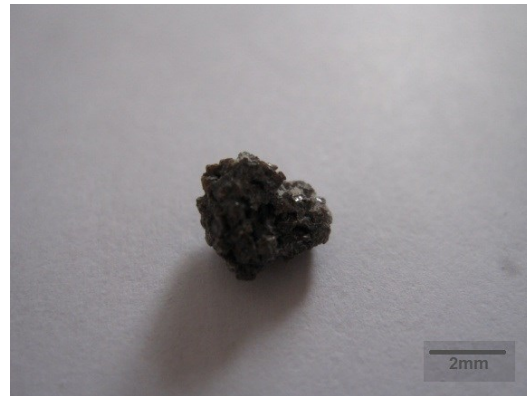
Fig. 22 "Normal" crystal size fused magnesia
