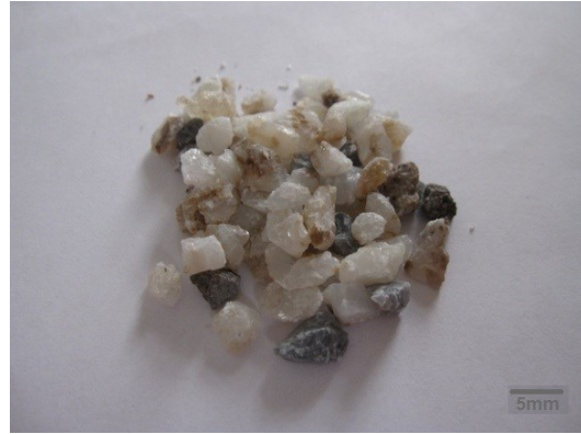
Fig. 25 Fused magnesia in residual group
