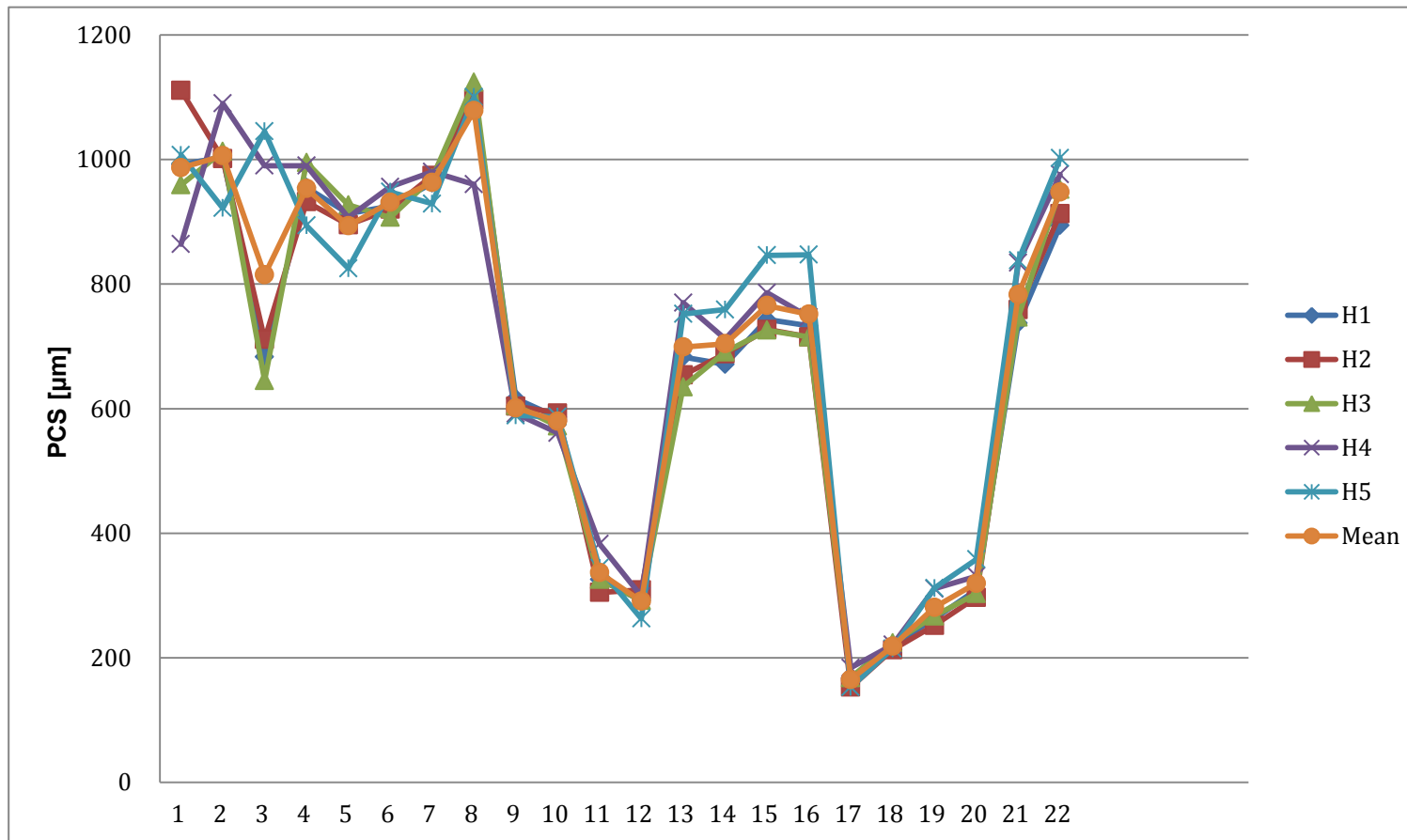
Fig. 30 Average periclase crystal size of portion < 1435 μm in [μm], from table 13 and 14
