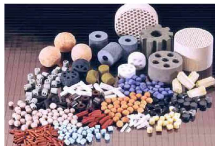
Figure 2.4: Examples of the various forms of shaped catalysts[19].
