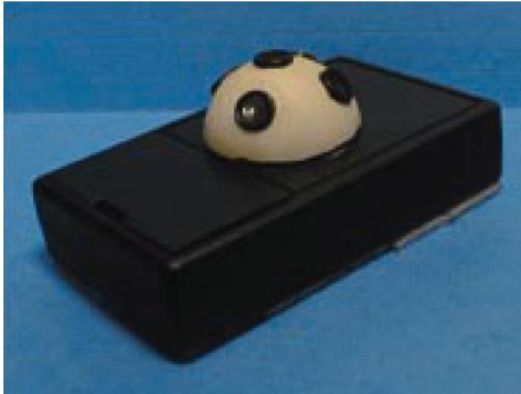
Abbildung 3.9: Active Bat Transmitter[WJH97]
