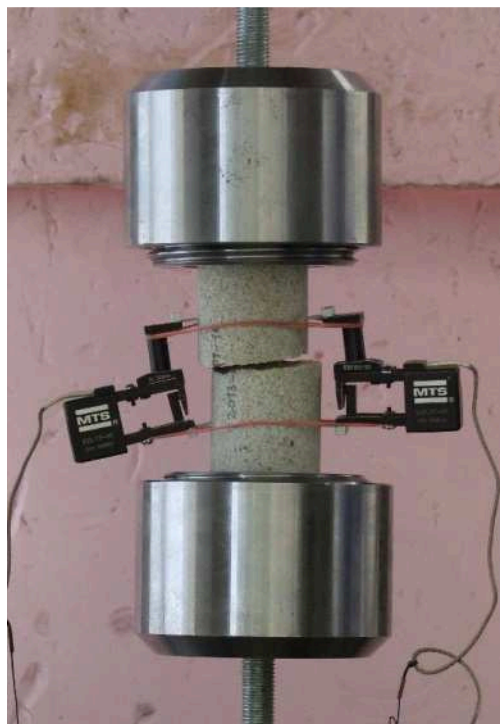
Illustration 7-2: Uniaxial tension test (11)
