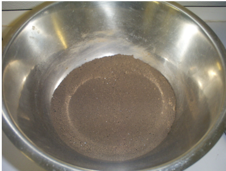
Figure 22.1 Homogeneous mixture of biocoal, electric arc furnace dust and CaO before watering and rotation
