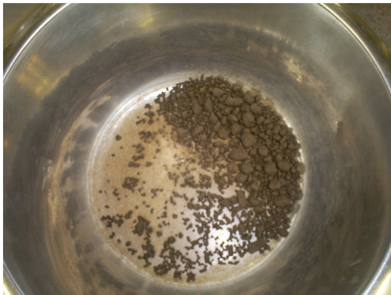
Figure 22.5 Large pellets produced by over watering the mixture or excessive drum rotation speed
