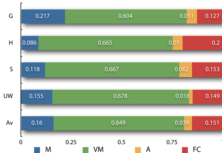
Figure 4.3 Proximate analyses of various types of biomass as received. Proximate analysis: ash yield (A), fixed carbon (FC), moisture (M) and volatile matter (VM) mass fractions ( \text{kg kg}^{-1} ). Types of biomass: G: grass/plant, H: husk/shell/pit, S: straw, UW: untreated wood and Av: average, [45]
