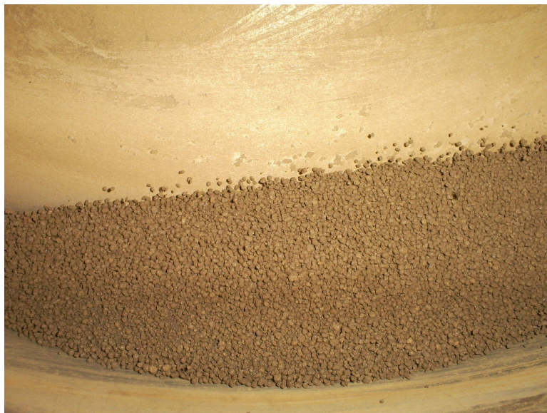
Figure 22.3 Pellet production: pellets being formed by the addition of water and by rotation of the pelletizer drum
