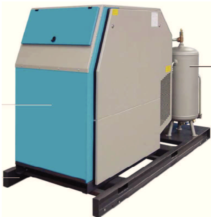
Figure 3.8: Compressor unit (Bauer Poseidon high pressure compressor, Verticus 5, Type HTA 120-4-5: operating pressure = 90-350 bar, F.A.D. = 5.4-7.1 m 3 /h)
