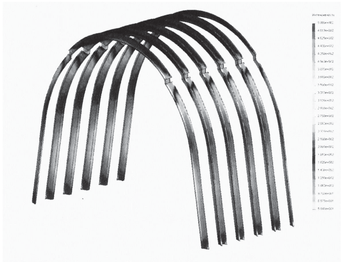
Figure 3.2. The diagram of reduced stresses in the arch support of the test model
