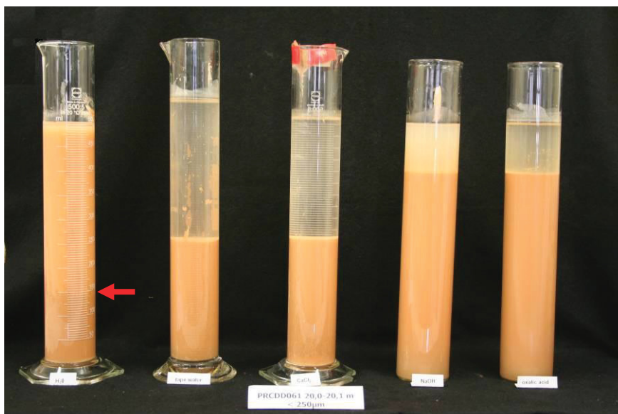
Illustration 71: Decantation test 3 from left to right sample in H 2 O, tap water, CaCl 2 , NaOH, oxalic acid
