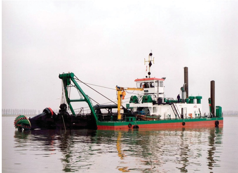
Illustration 16: IHC Beaver Cutter Suction Dredger 6518 C
