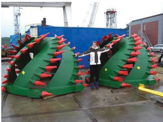
Illustration 23: Cutter head with teeth
