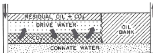
Figure 9: Simultaneous injection of CO 2 and water process
