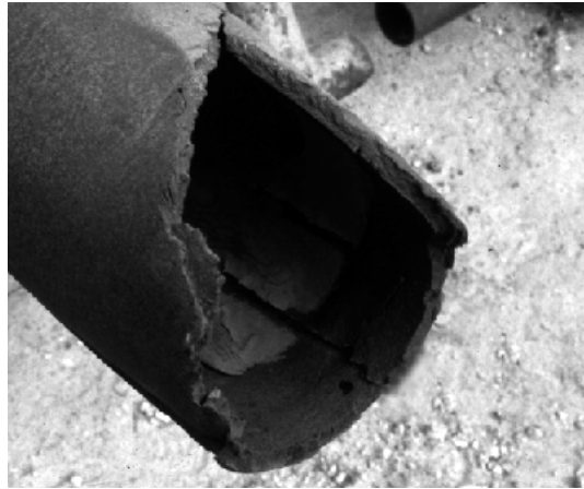
Figure 4-8: Combined load failure with helical shape fracture [29]
