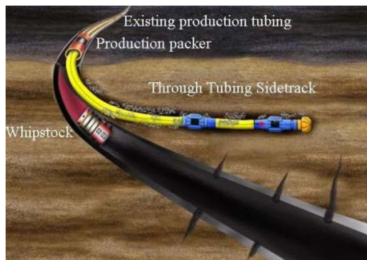
Figure 5-1: Principal of Through-Tubing Rotary Drilling [61]
