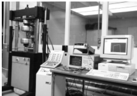
Figure 6-1: Fatigue testing machine (compressive and tensile loads) [19]
