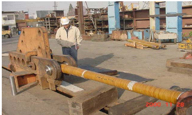
Figure 9-2: 10 ft full diameter tension test [57]
