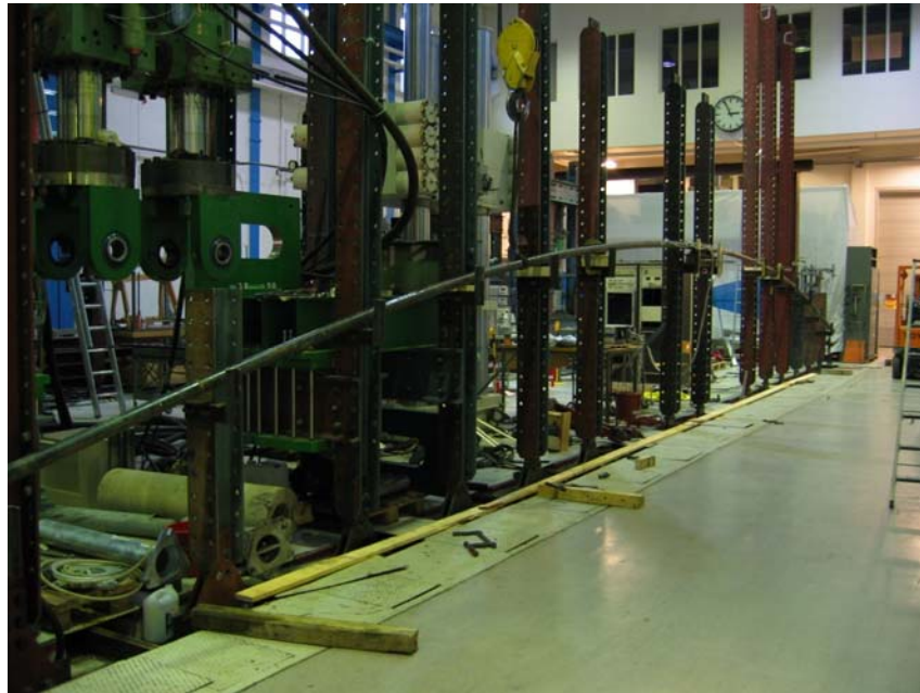
Figure 6-3: 50° dogleg bending test [62]
