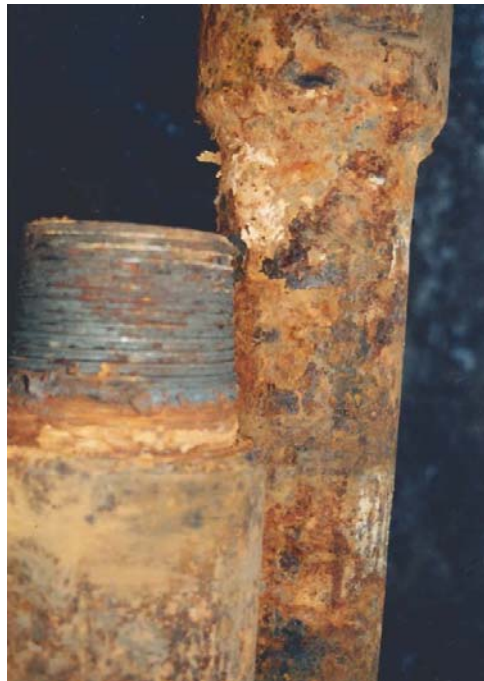
Figure 4-10: Effects of corrosion on drillpipes [62]
