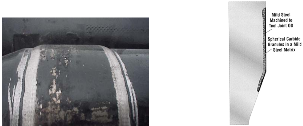
Figure 2-1: Raised, smooth [62] (left) and flushed [2] (right) hardbanding on tool joint
