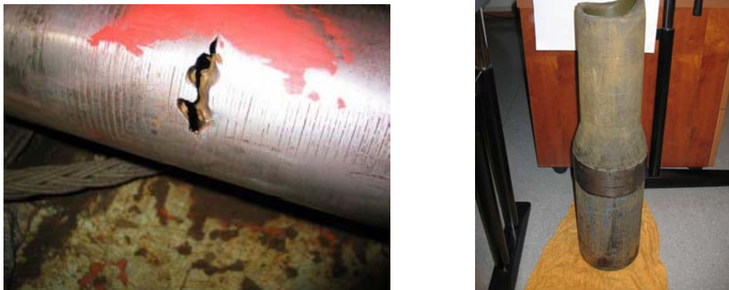
Figure 4-1: Washout on drillpipe [8] (left) and broken pipe [62] (right)
