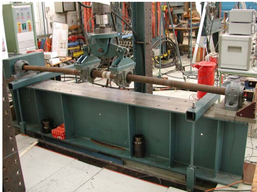
Figure 6-4: Rotating bending test for 2 7/8" drillpipe [62]
