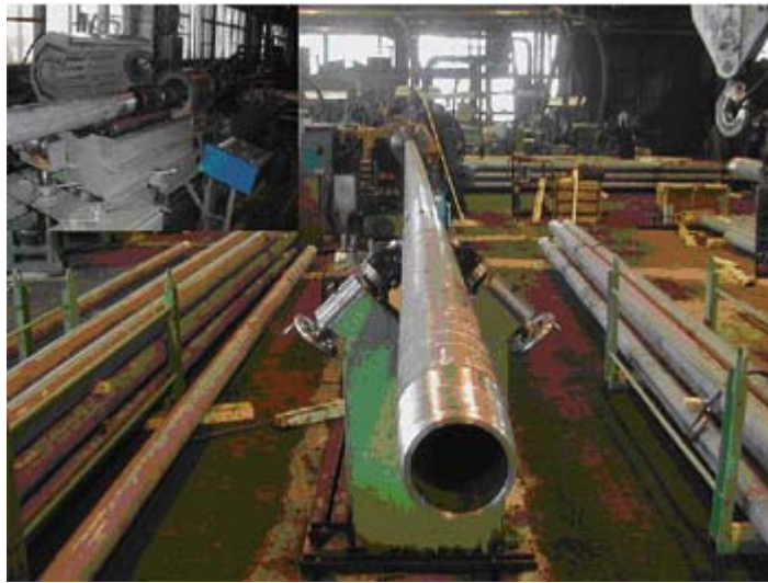
Figure 9-1: The Serov Mechanical Plant assembles steel tool joint-aluminum pipe, (top left) [53]
