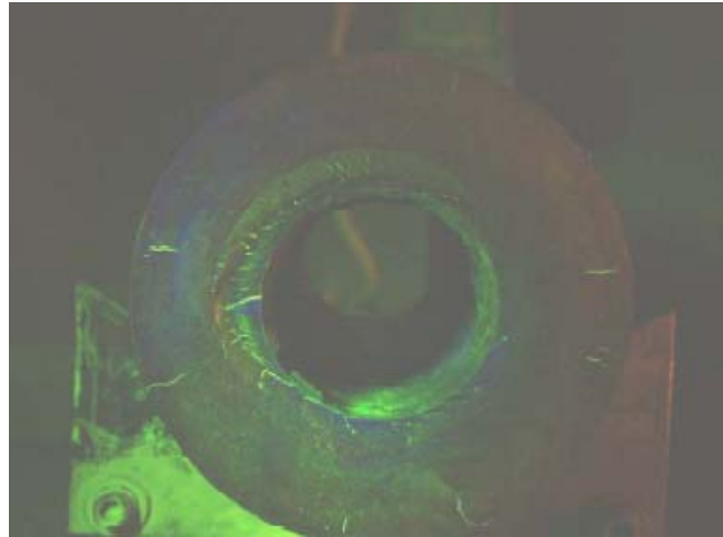
Figure 8-1: Wet fluorescent magnetic particle image of a fracture surface with cracks originating from ID and OD [13]
