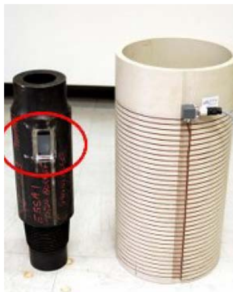
Figure 7-13: Tag integrated in the tool joint (right) and the reading/writing antenna (left) [40]
