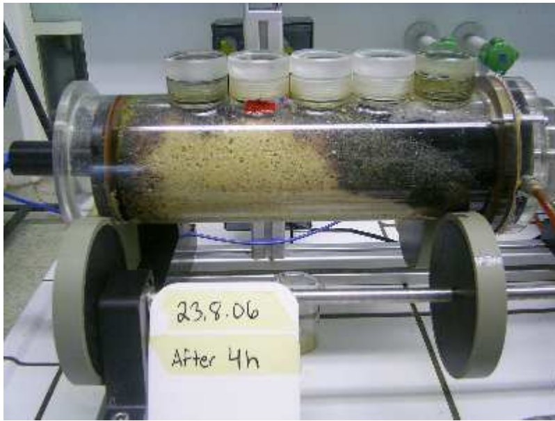
Picture 3: First horizontal transport system with integrated oxidant solution circulation
