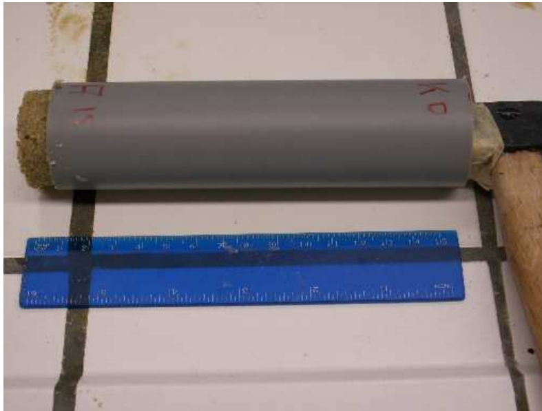
Picture 5: Pushing out the soil column in order to produce slices for analysis
