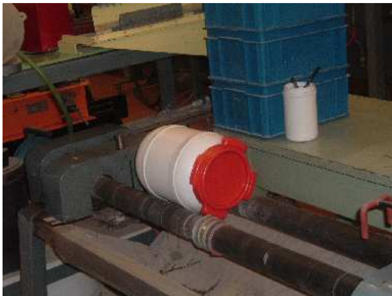
Picture 2: Mixing of spiked soil
