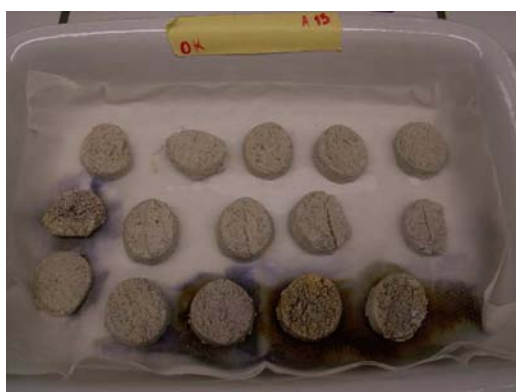
Figure 30: Analysis of horizontal transport experiments with peroxodisulfate spiked soil
