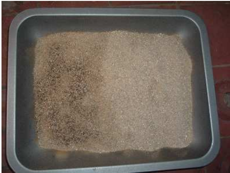
Picture 1: Soil spiking with diesel oil
