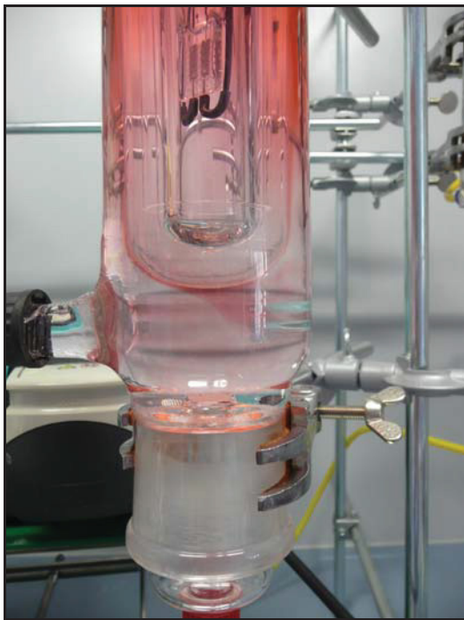
Figure 8.7: Step tracer test in large PFR: two flows in fluid visible (deep and light rose)
