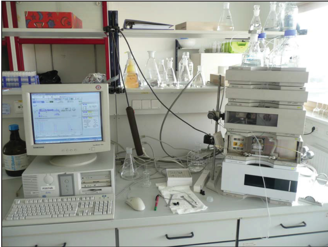
Figure 7.2: HP 1100 Series HPLC instrument used to EDTA concentration determination
