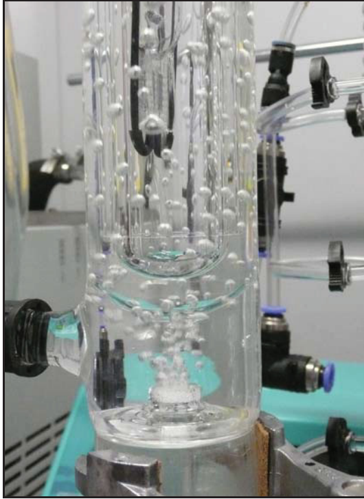
Figure 9.6: Air bubbles in small pipe reactor
