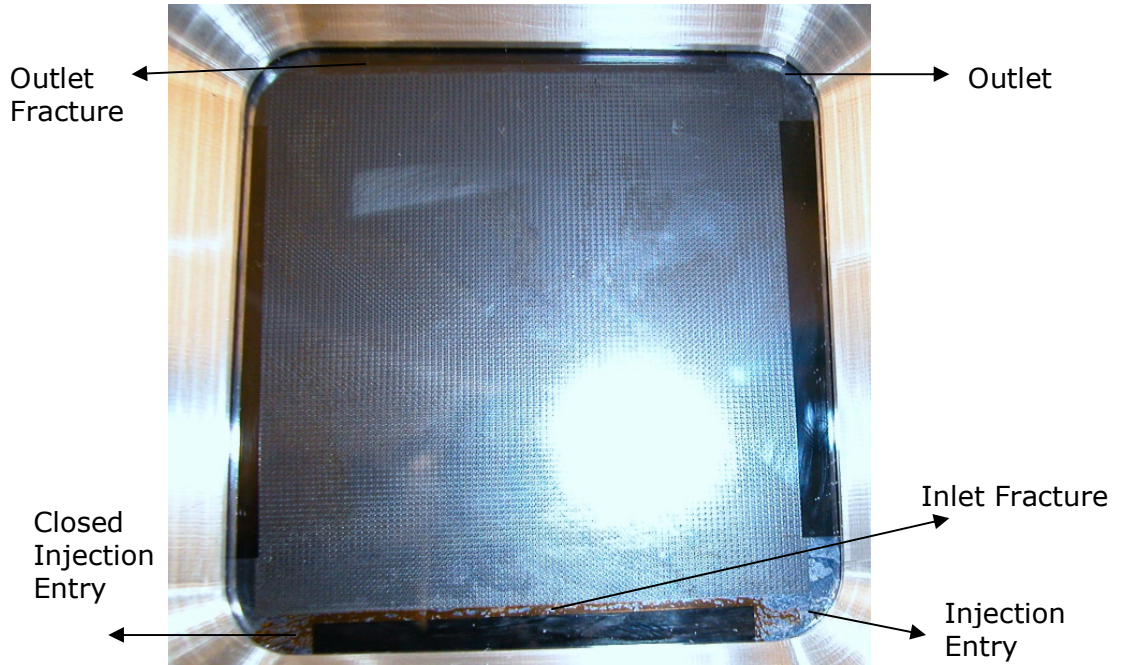
Figure 44: The inlet and the outlet fractures of the micromodel, meso scale. (Inlet fracture is being filled with the oil)
