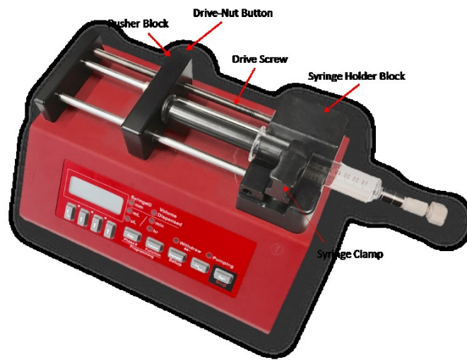
Figure 3-9 – NE-300 syringe pump and its major components
