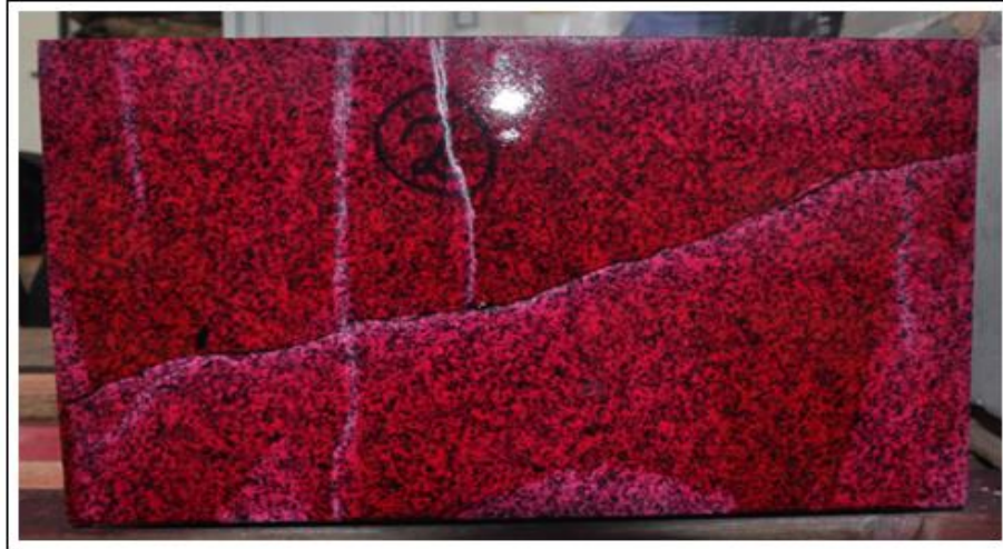
Figure 4 - 6: Block #2, radiated time 45 sec, side cracks
