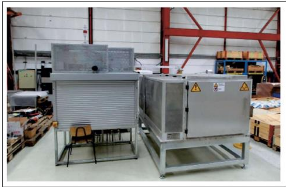
Figure 3 - 1: The microwave facility (Magnetron and control unit on right side and safety cavity – left side)
