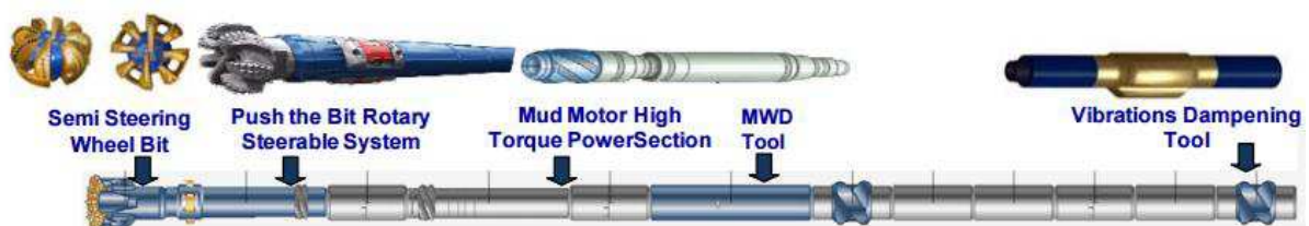
Figure 18: Redesigned BHA which improved drilling time for 300%.
