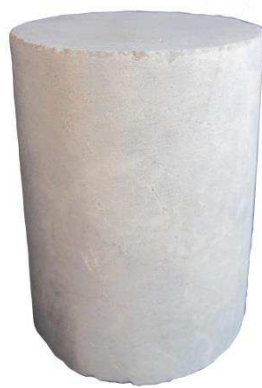
Figure 22: The overcored limestone sample which was used in the experiment.
