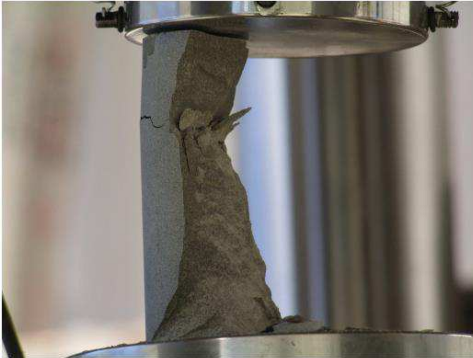
Figure 38: The sandstone breakage.
