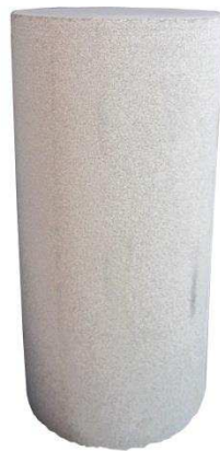
Figure 25: The overcored sandstone sample which was used in the experiment.
