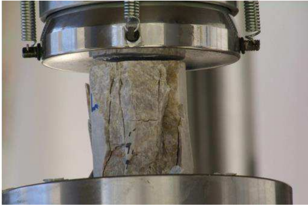
Figure 35: The limestone breakage.
