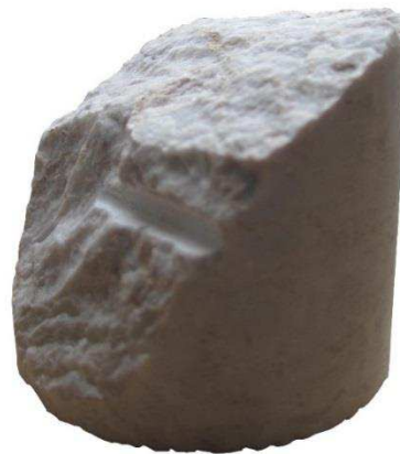
Figure 24: The broken part of the limestone sample. Foliation where the sample broke is clearly visible.
