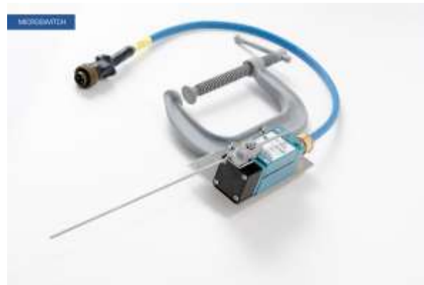
Figure 21: Stroke counter for mud pumps [54]. The blue cable stands for Ex i, where at a possible spark, the spark energy is below the ignition energy of the surrounding explosive area.
