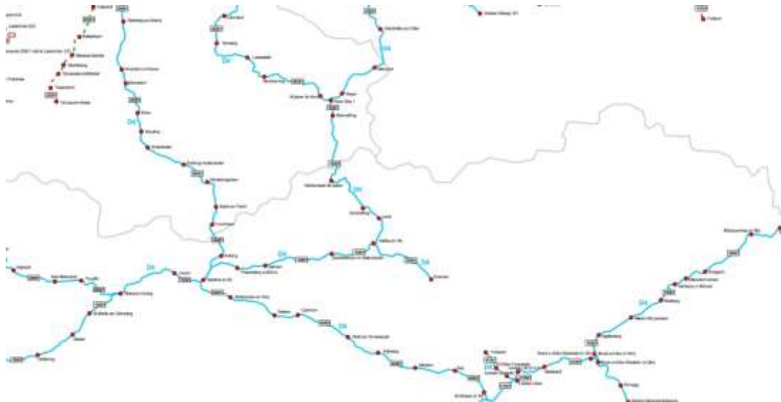
Figure 58: Cut-out of rail road network load classes. The blue lines are D4 load classes which stand for 22.5 t axel load and 8 t / m meter load.
