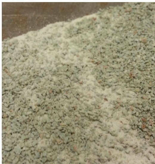
Illustration 4-18: Salt abrasion of Multi 5 S.
