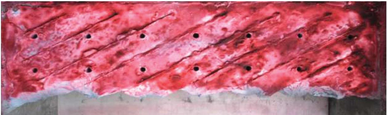
Figure II-41 JS3 Alpha top view after blasting of 1 st row
