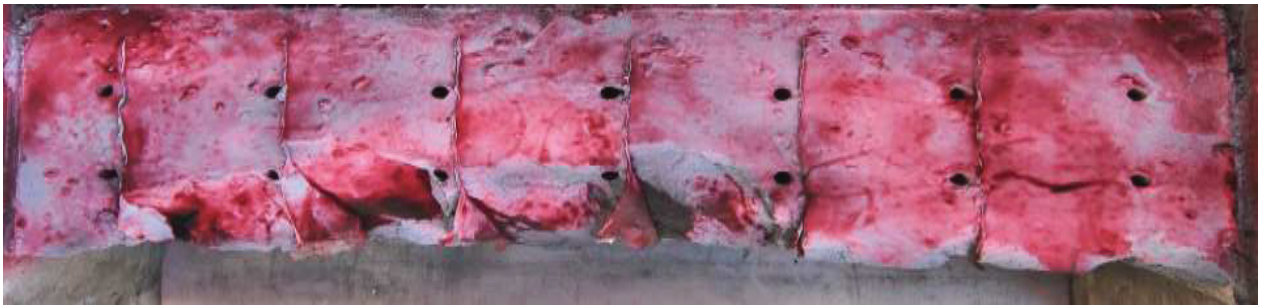
Figure II-56 JS4 Alpha top view after blasting of 1 st row
