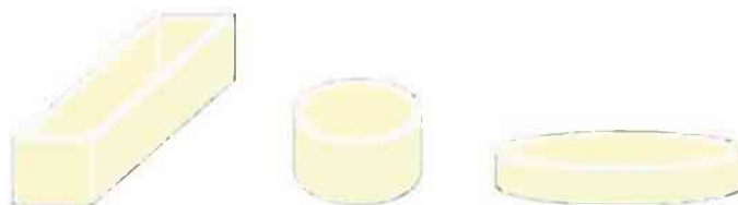
Figure 3–4: Crucible geometries for rectangular (left), cylindrical (middle) and concentric (right) samples.
