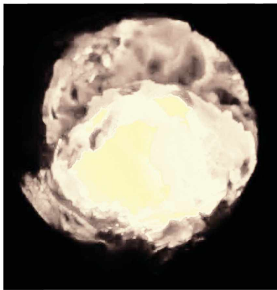
Figure 4–5: Slag incrustation of the crucible for 3.5 wt.-% manganese.
