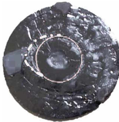
Figure 3–8: Unevenly distributed supporting points and decentralised melting pool .
