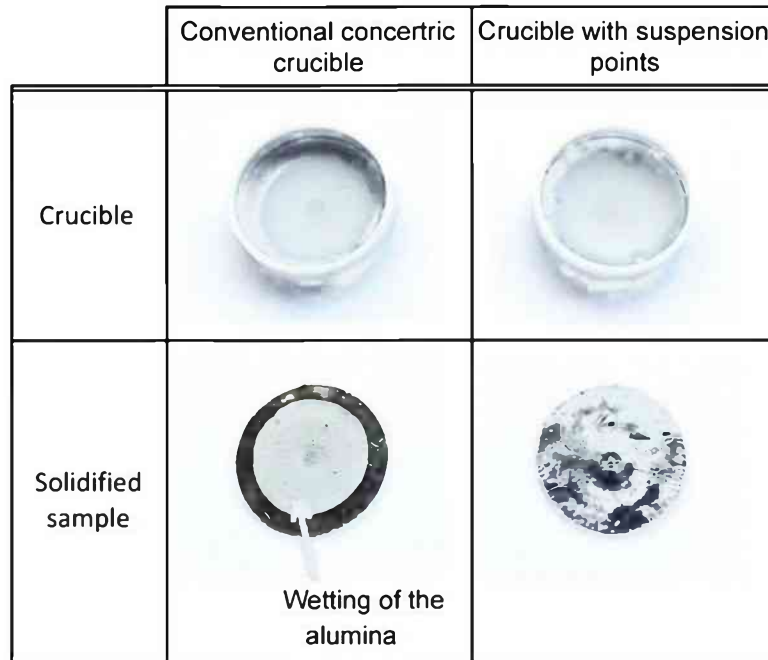
Figure 3–7: Comparison of the conventional crucible and the newly developed crucible with suspension points.
