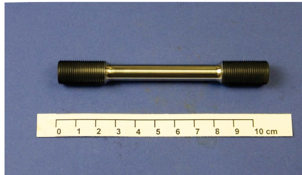
Figure 3.2: Used sample geometry for tensile tests.
