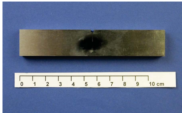
Figure 3.3: Dimensions of the used SENB samples for fracture toughness measurements.
