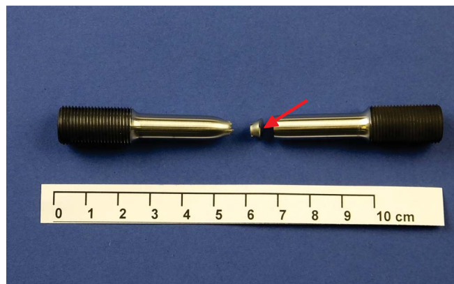
Figure 4.37: Fractured tensile test sample. The arrow indicates the position of XRD analyses.
