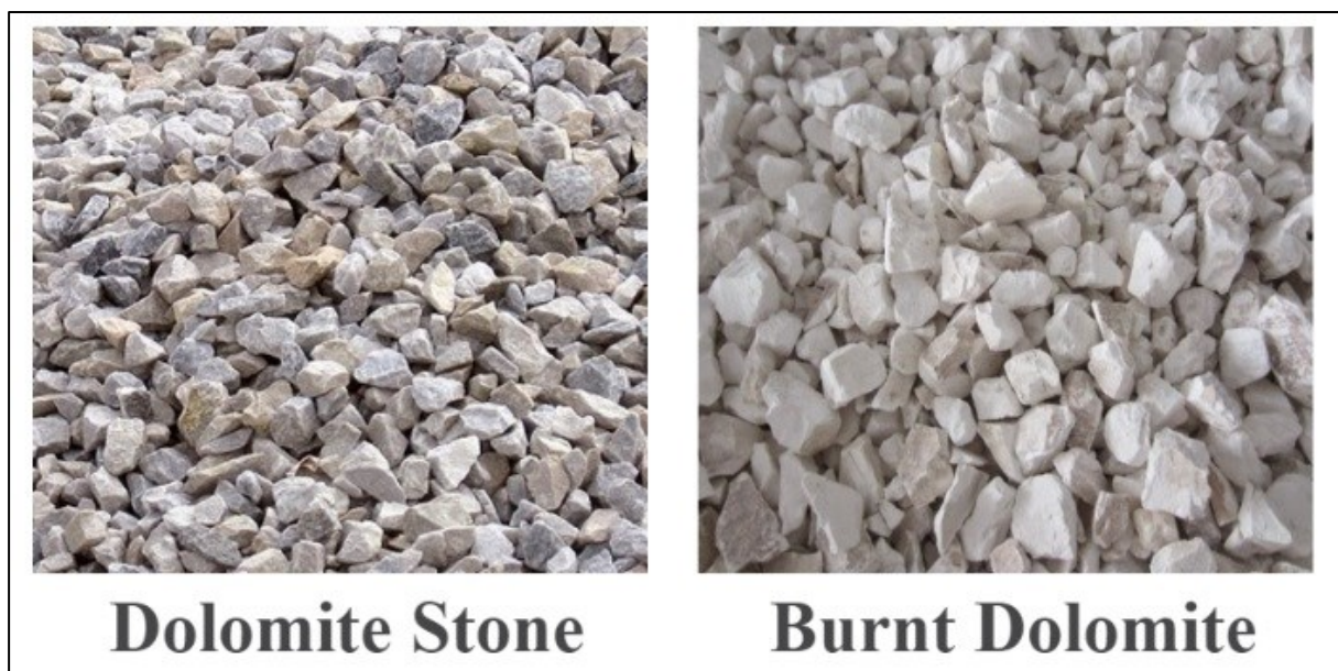
Figure 2-2: Comparison of dolomite stone and burnt dolomite [33]
