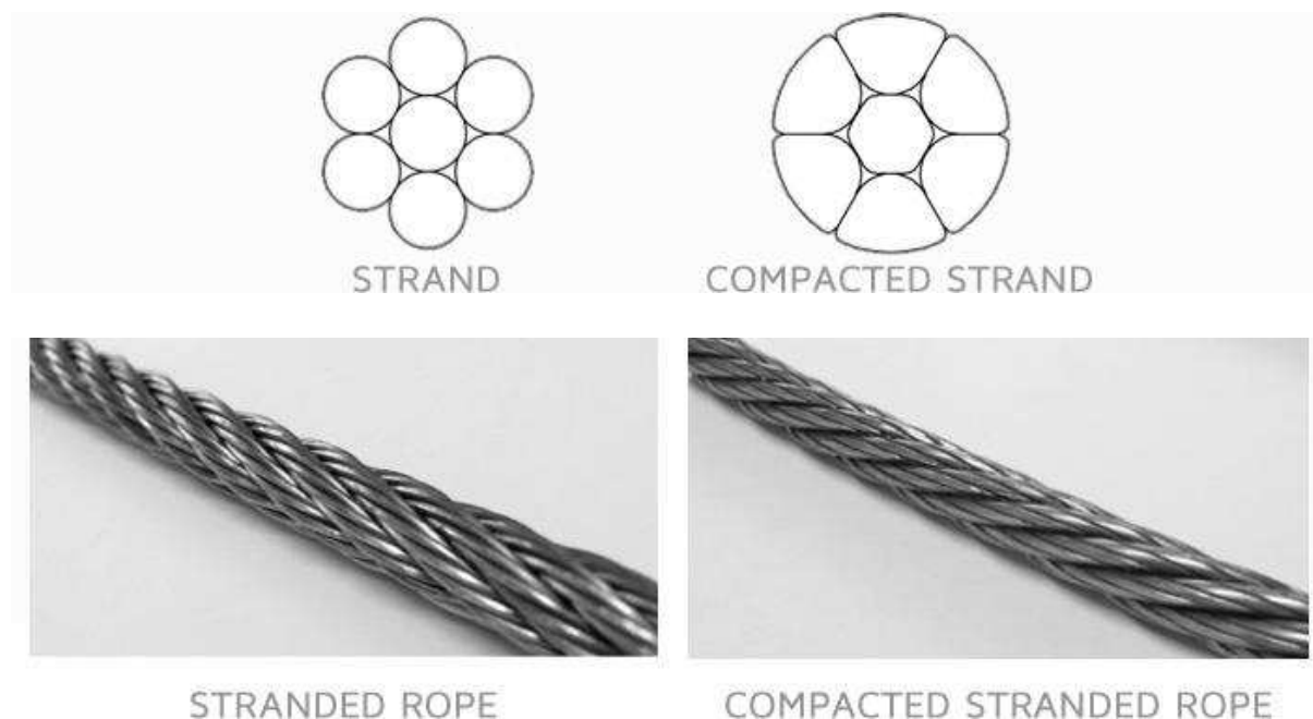
Figure 21. Comparison between stranded and compact strand wire ropes [28]
