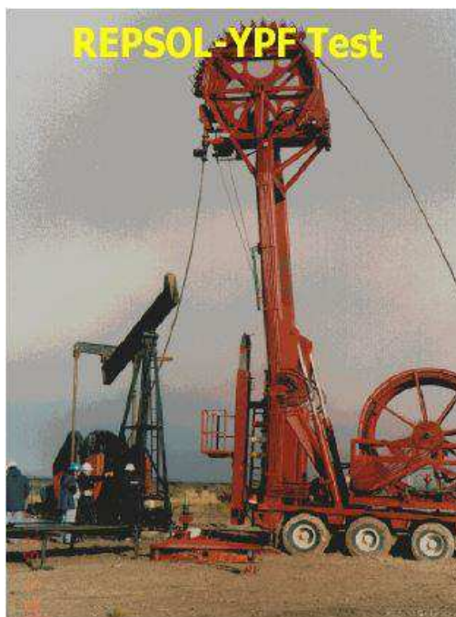
Figure 10. CT Pump Test in Argentina [18]
