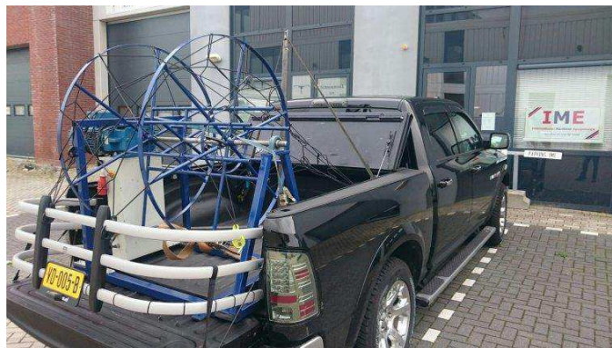
Figure 39. A typical synthetic rope spooling setup [48]
