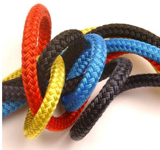
Figure 27. Example of braided ropes [40]
