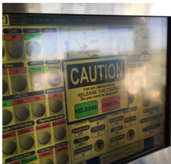
Fig. 25 – Driller's control dashboard displaying casing release override.
