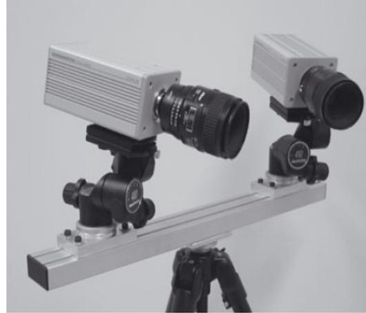
**Fig.14: Binocular stereovision [41]**
