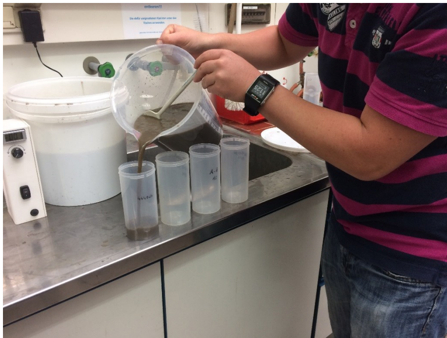
Figure 10: Filling the beakers with a well homogenised slurry sample
