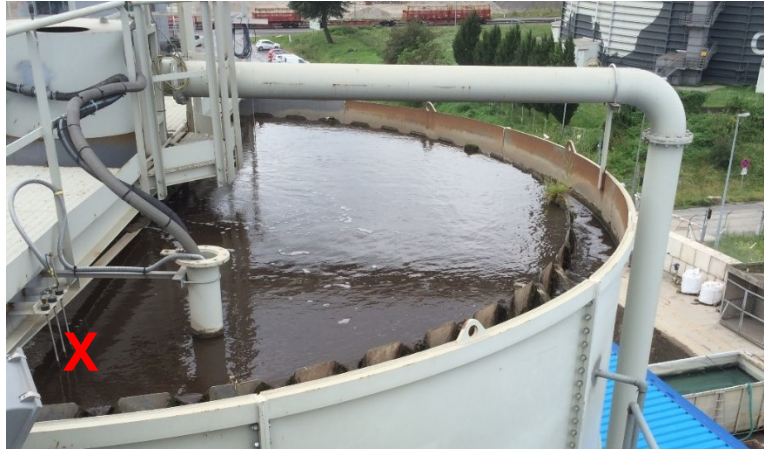
Figure 23: Sampling point of the thickener overflow. On the picture, only the new thickener is visible.
