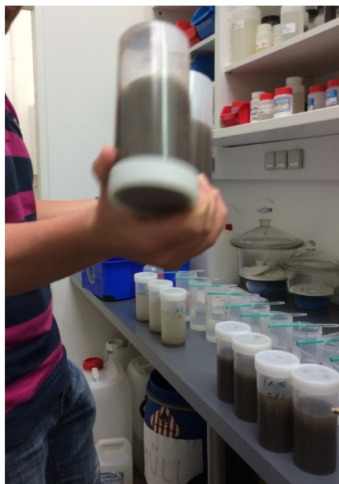
Figure 13: Shaking the glasses with two strong shaking movements
