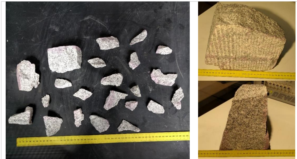
Figure 3.4-2 Pieces, created as a result of failure of the sample
