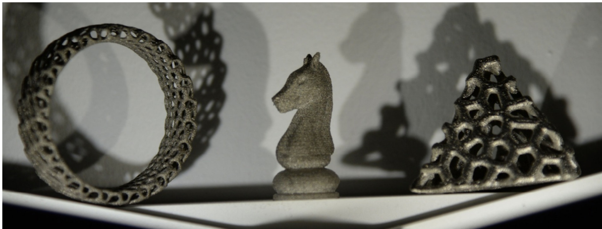
Figure 1.1: Titanium parts manufactured by 3D printing methods (© Dominik Hammerer)
