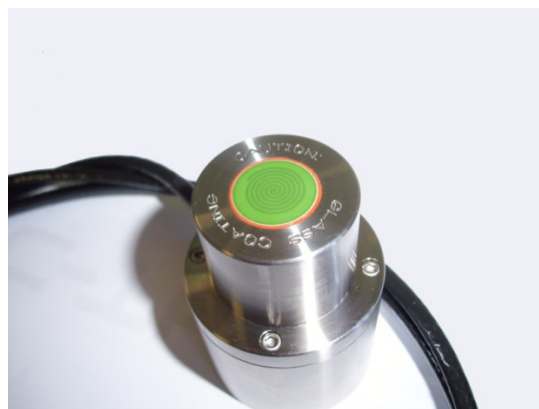
Abbildung 19 Modified transient plane source – Sensor [120]
