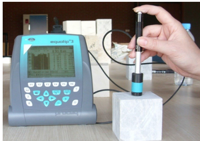
Figure 31: Surface hardness tester (Yilmaz et al. 2015)
