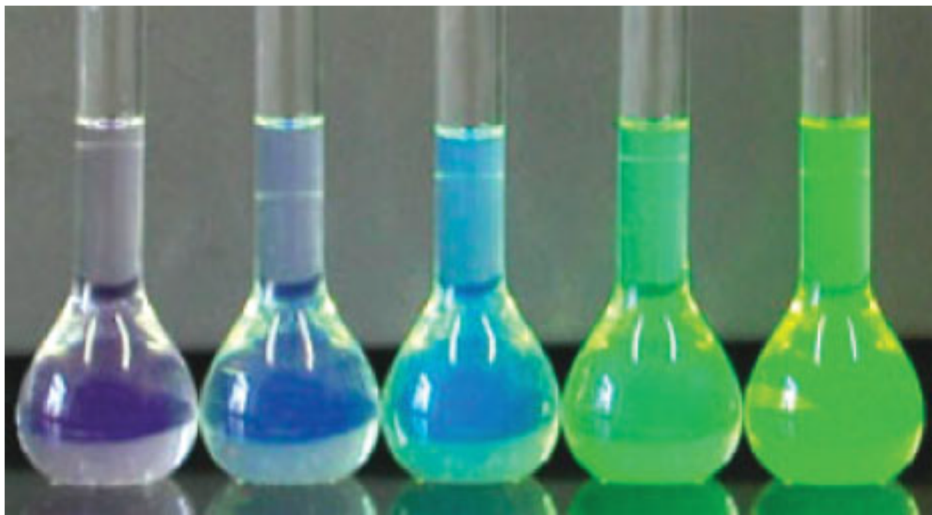
Figure 1: The difference in emitted wavelength for the fluorescence, dependent on the size of the nanoparticles is shown for CdSe-NCs, with the diameter increasing from left to right. Ref. [3]
