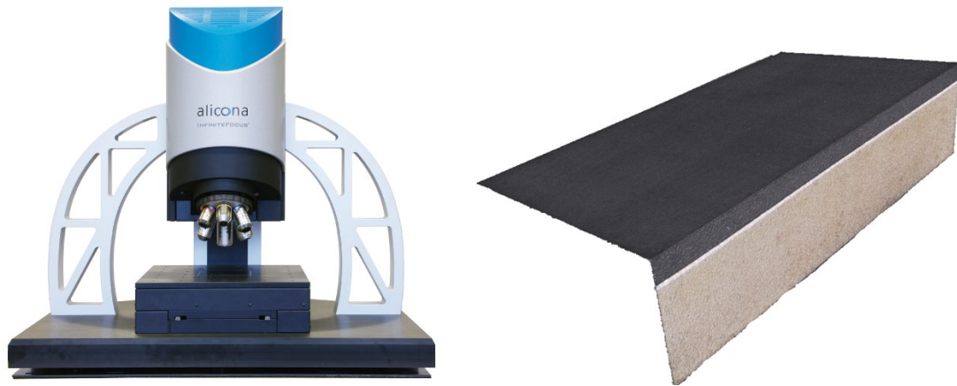
Figure 40: Alicona™ measurement equipment (left) and a visualisation of a carbide backed PCD to verify the 90° angle left
