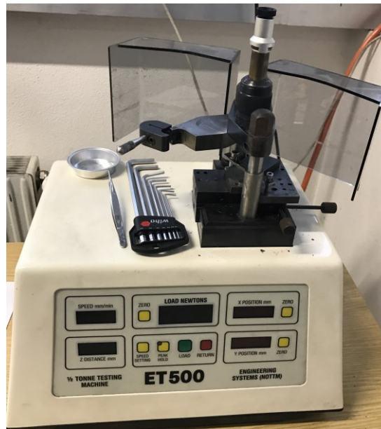
Figure 38: ET500 testing machine for edge toughness tests
