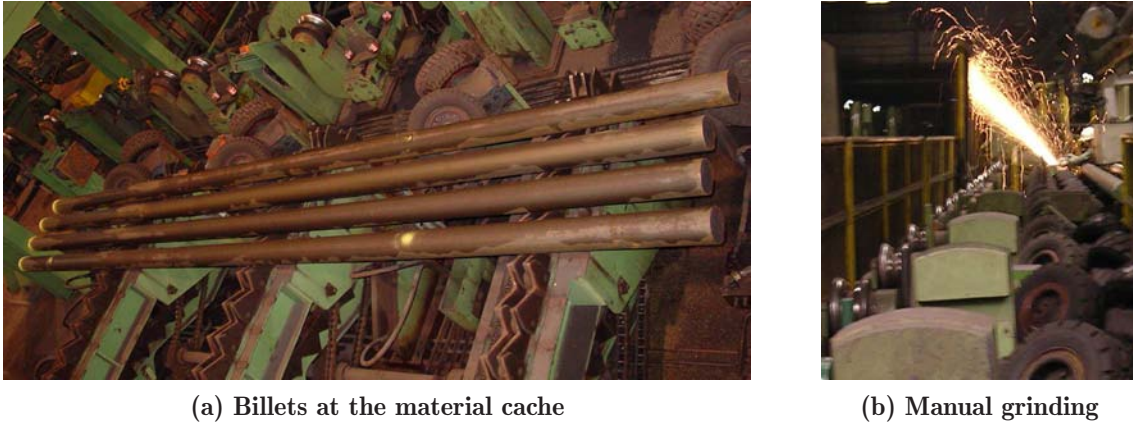
Figure 1.1: Figure (a) shows four circular billets at the material cache, which separates the continuous operating Thermomatic inspection from the subsequent machining process. The frontmost billet exhibits two color markings that indicate the presence of surface flaws. The image to the right (b) depicts the manual grinding process.
