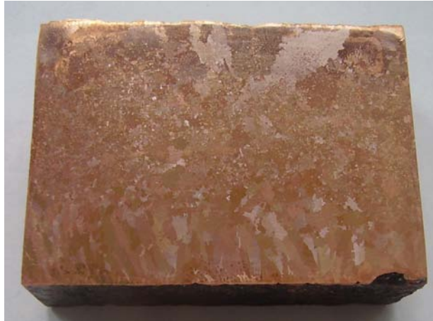
Figure 93: Macrostructure of anode I (new cathode copper mould, new cooling arrangement)
