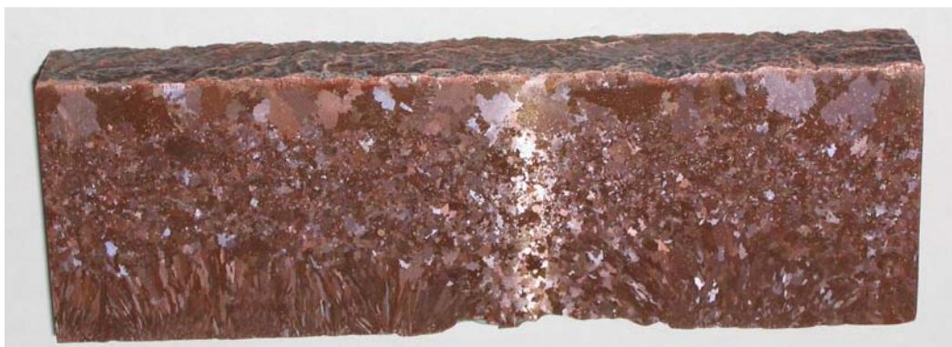
Figure 90: Macrostructure of anode H (new cathode copper mould)
