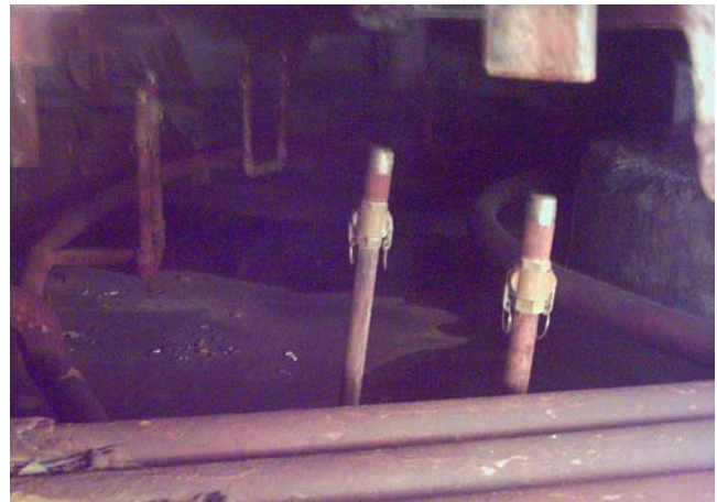
Figure 46: Water spray cooling on the air side (left) and the mould bottom (right)
