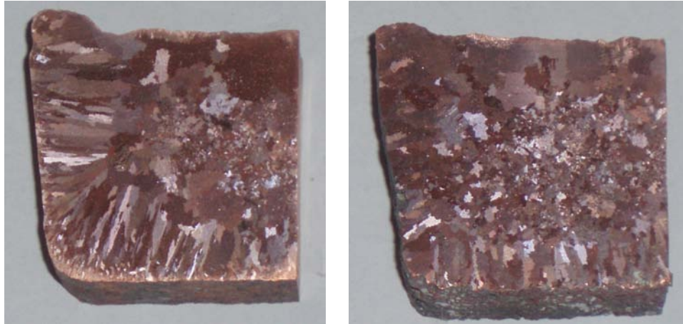
Figure 89: Outer area of anode E (carbon black, left) and F (barite, right)
