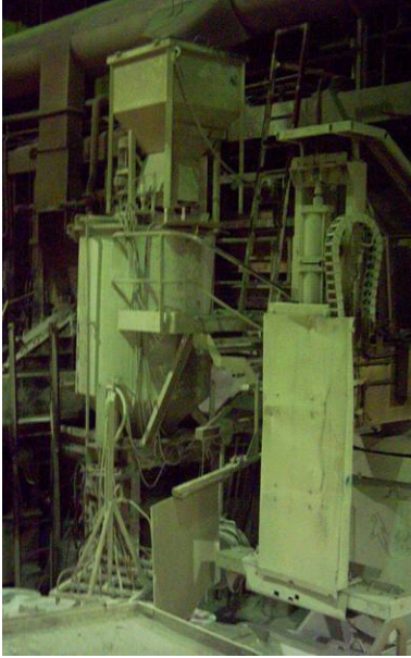
Figure 44: Automatic mould wash application
