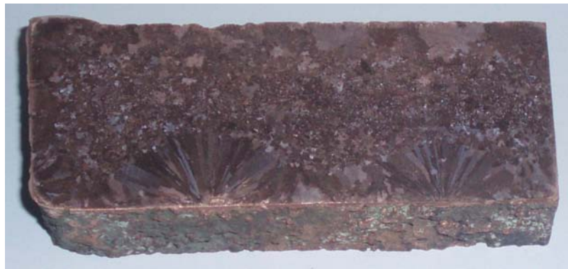
Figure 97: Fan-shaped columnar crystals in sample 2.5 (anode A)
