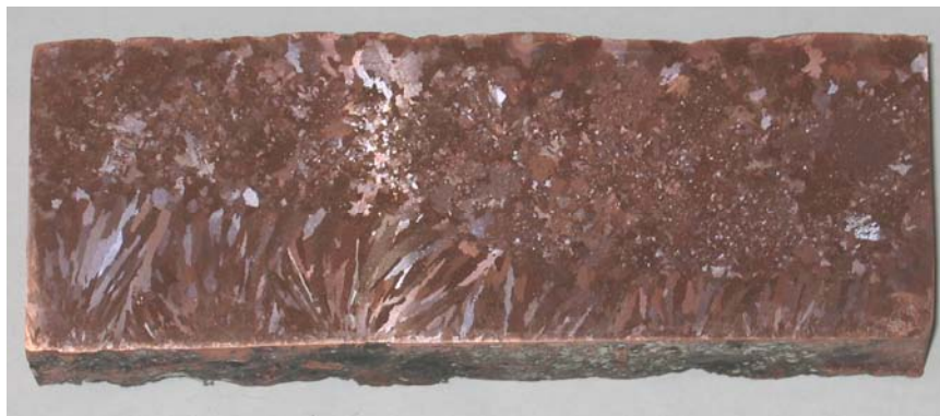
Figure 92: Macrostructure of anode G (mould with cooling ribs, type 1)
