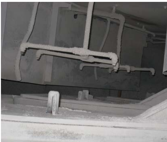
Figure 46: Water spray cooling on the air side (left) and the mould bottom (right)
