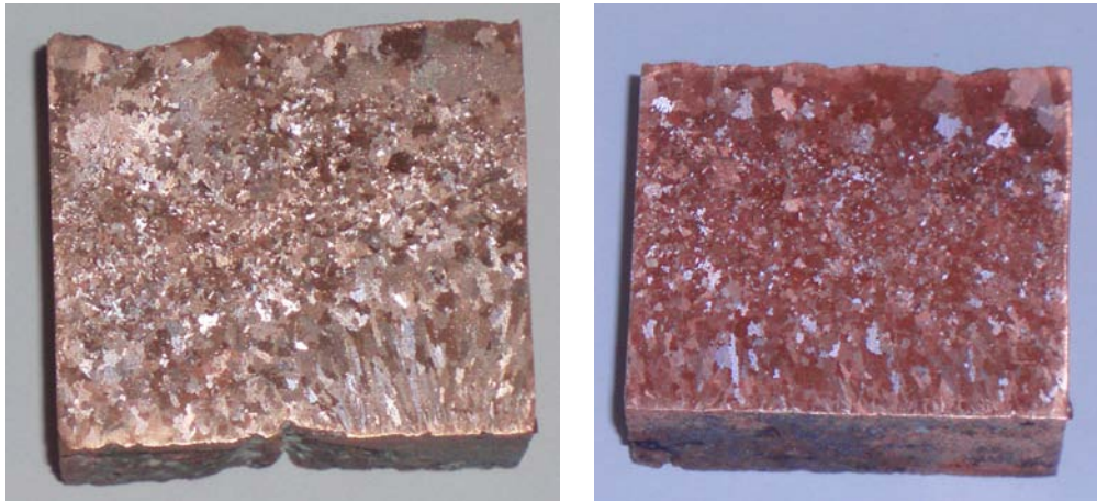
Figure 88: Structural variations under different cooling conditions (mould wash)—anode F (barite, left) and E (carbon black, right)
