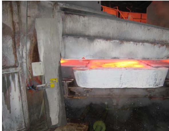
Figure 53: Infrared mould surface temperature measurement
