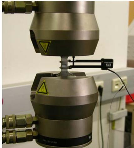
**Fig. 4.9:** Testing setup for strain controlled LCF experiments
