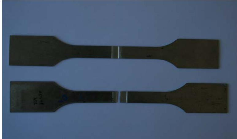
**Fig. 5.23:** Welded tensile specimens (direction of the weld perpendicular to the specimen axis)
