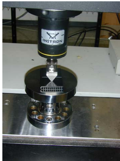
Fig. 1: Indentation test set-up with a prismatic indenter applied to the absorber sheet specimen.
