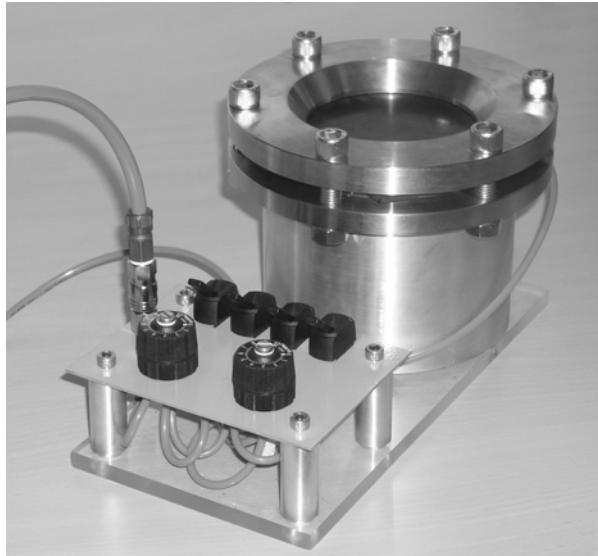
Fig. 1. Biaxial tensile test device also showing the specimen fixed between the two clamping devices
