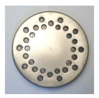
Fig. 1: Cr mosaic target with circular blind holes for WS<sub>2</sub> and Cr inlays used for coating deposition.
