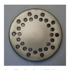
Figure 5.2: Cr-target used for deposition of coatings within the system Cr-MoS<sub>2</sub>-N and Cr-WS<sub>2</sub>-N.
