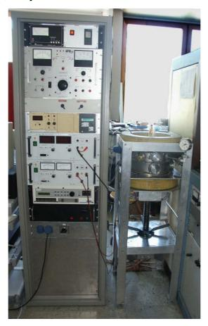
Figure. 5.1: Picture of the PVD system used for coating deposition.
