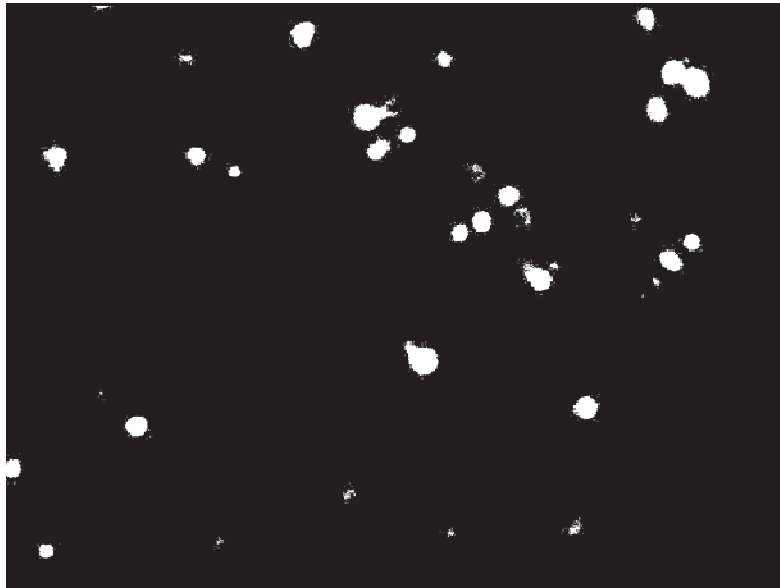
Figure 114: Exemplary picture of particle distribution within 2mm*2mm image region of filter fibre sample. Particles glow under influence of laser light. The closer to focal plane, the sharper the individual particle image becomes.
