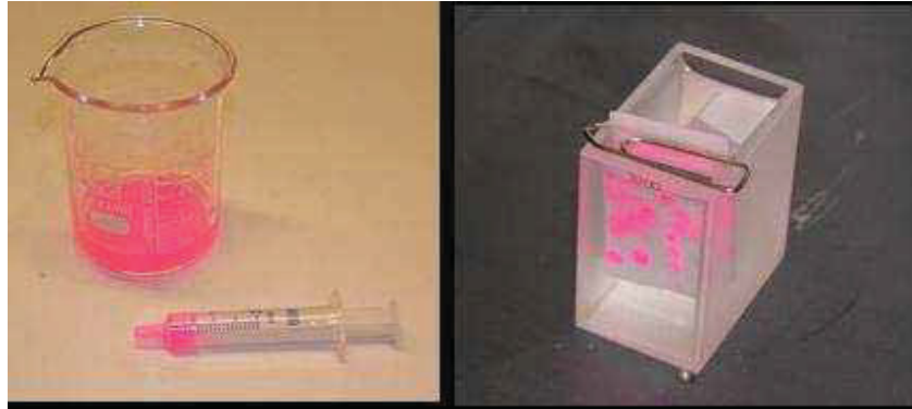
Figure 108: Rh-B marked PMMA particles in oil dispersion (left) and on filter fibre sample (right).
