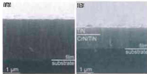
Fig. 5: SEM fracture cross sections of the multilayer CrN/TiN coating prepared with one fold rotation at a substrate temperature of 450 °C using a UBMS power at the Ti cathode of 4 kW (a) and adding a TiN top layer prepared by UBMS with 4 kW (b).
